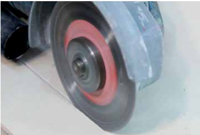
Example of variable speed grinder using diamond electroplated blade to make straight line cut out
