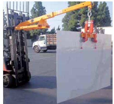
Example of forklift boom & pinch clamp
