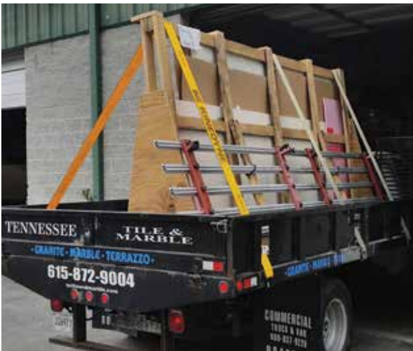
A-frame properly strapped to open truck
